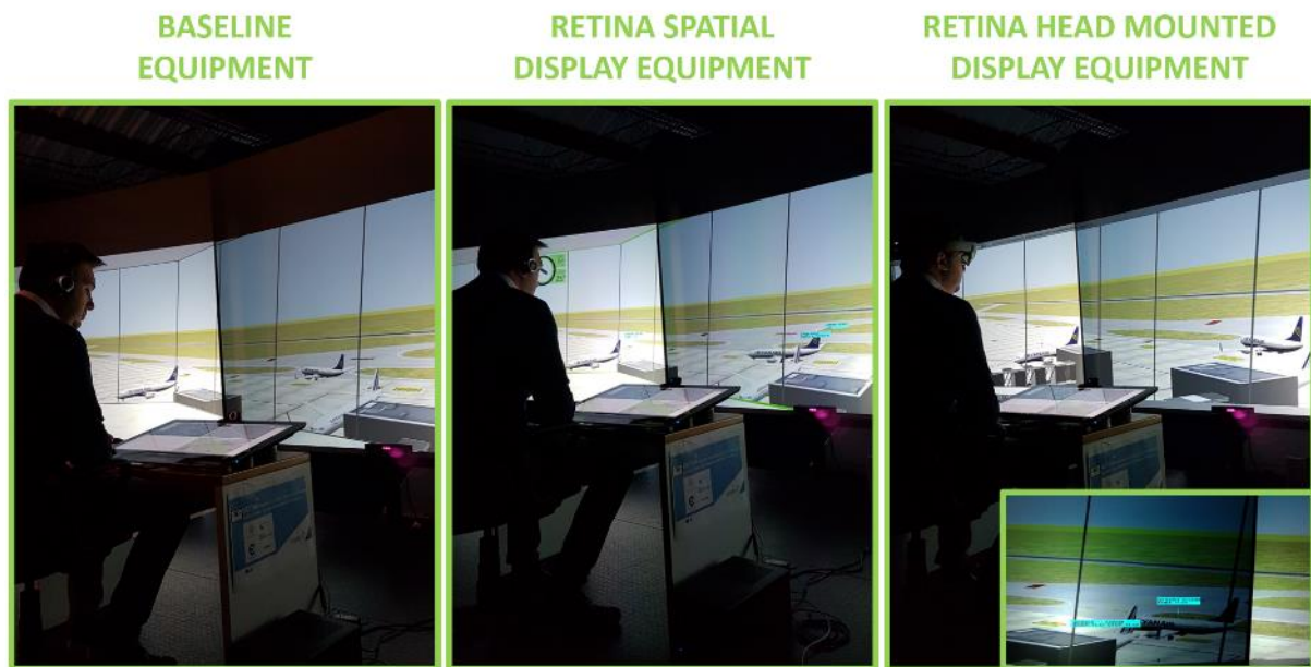
Figure 4 RETINA Validation Platform. The AR App derives the relevant Augmented Reality Overlays and deploys them on the appropriate ATCO Head-Up Interface (being either Spatial Display or Head Mounted Display). The baseline equipment serves to compare data obtained vs success criteria and validation targets identified below.
